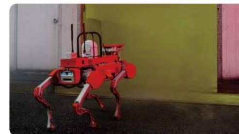
It goes into extreme environments such as toxic, hypoxia, collapsed buildings to operate detection, rescue, supplies transition, also it helps to reduce the occurrence of secondary
